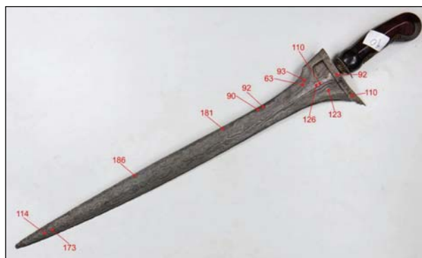
Figure 1: Photograph of kris N 32590, with locations and corresponding results of hardness measurements.
