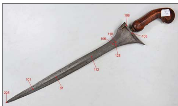
Figure 3: Photograph of kris N 32592, with locations and corresponding results of hardness measurements.
