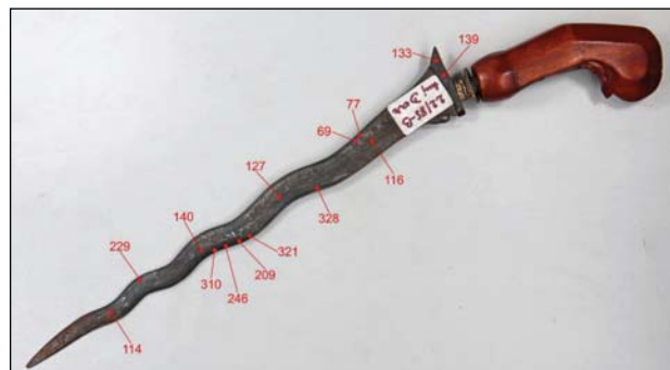
Figure 6: Photograph of kris 22/85–B, with locations and corresponding results of hardness measurements.
