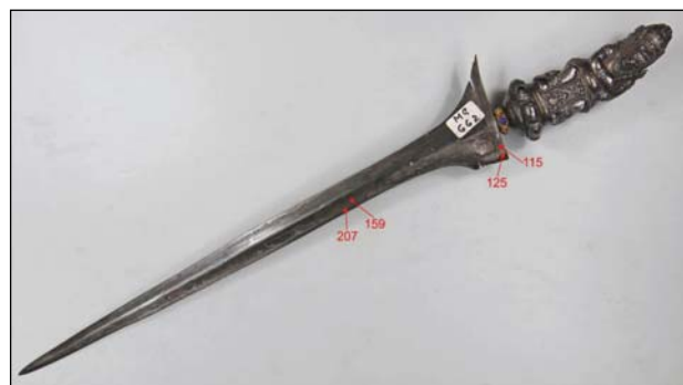
Figure 4: Photograph of kris MG 662, with locations and corresponding results of hardness measurements.
